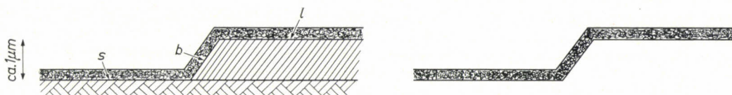
Fig. 1. When the surface of a thin film is scratched with the point of a razor blade, a fairly clean fracture surface b is obtained at some places. A continuous replica can now be made of the film surface l , the fracture surface and the exposed surface s of the substrate. The step-like replica can be detached without damaging it.
