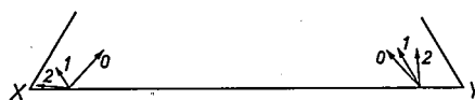
Fig. 22. Initial slopes of the boundaries of a miscibility gap calculated [6] for (b - c)/a = 0, 1 and 2 , indicated by the arrows 0, 1 and 2 respectively.
