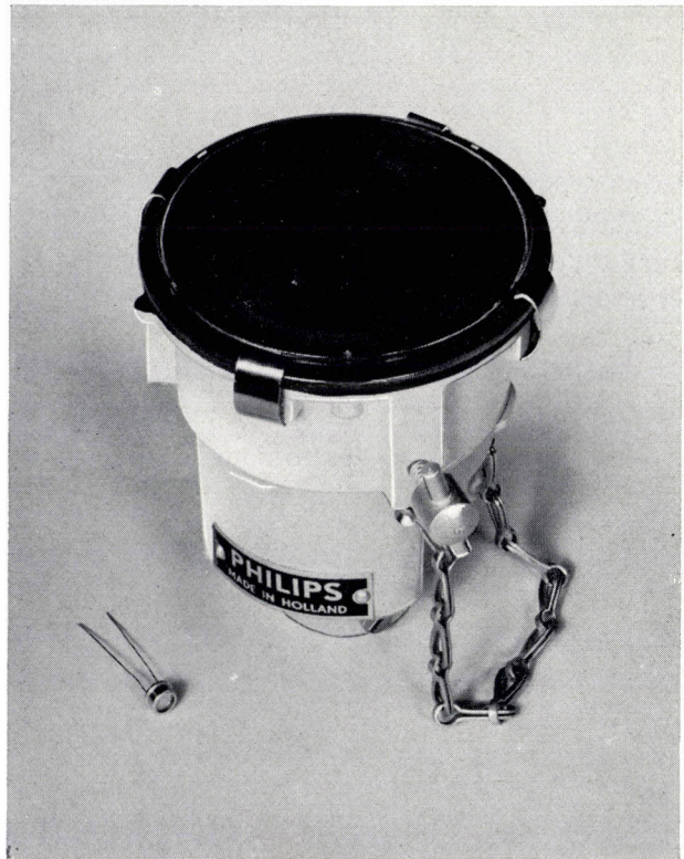
Fig. 16. Fitting in which the resistor combination R_1 (see fig. 14) is placed. To prevent it from being obscured by snow, the fitting is provided with heating controlled by a thermostat. A light-sensitive resistor is shown in the foreground.
