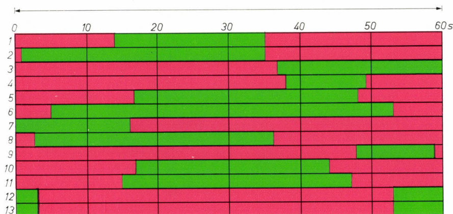
Fig. 2. Bar diagram of an optimum traffic-light sequence calculated under specified conditions for the intersection of fig. 1.
