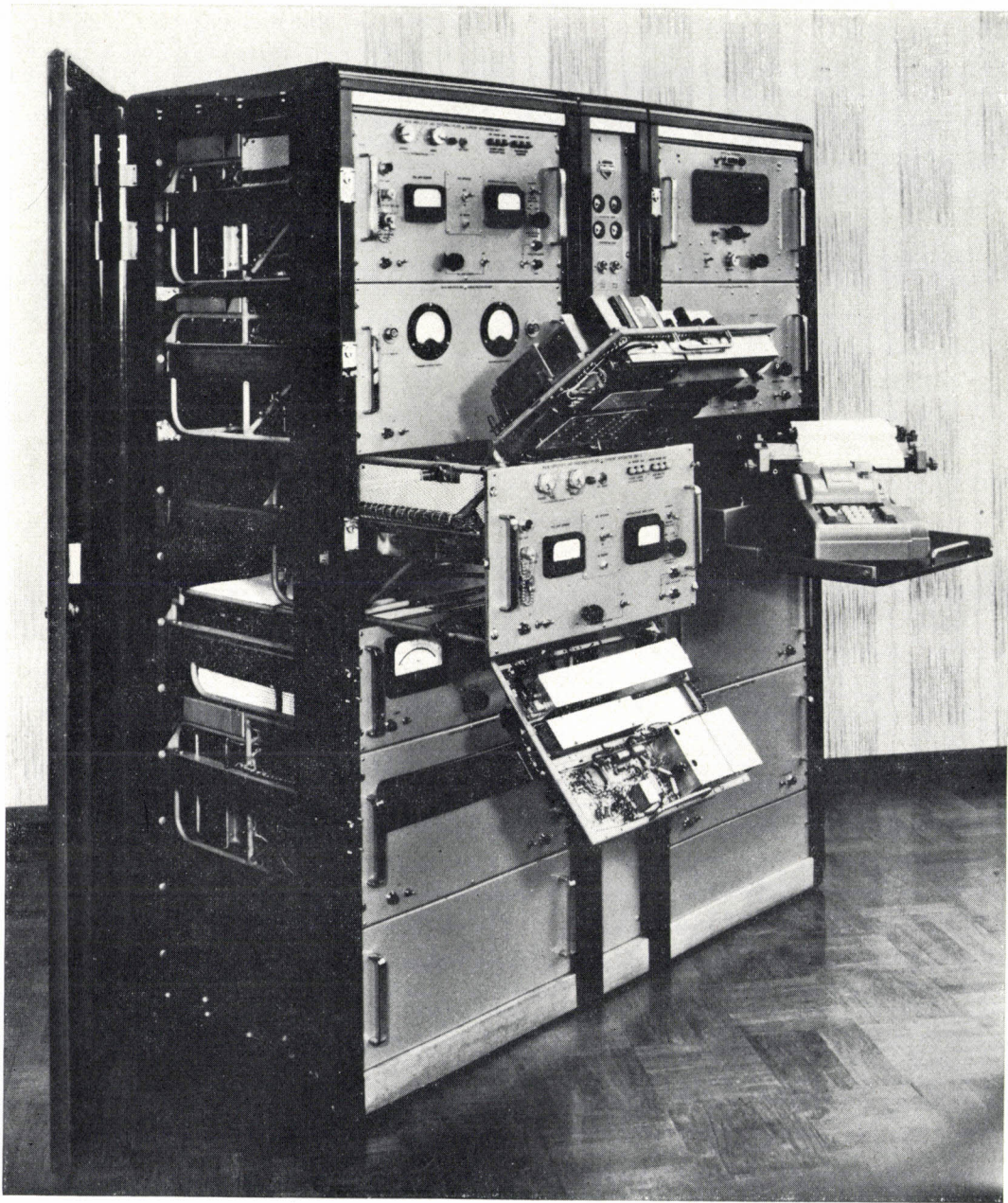
Fig. 10. The correlator. In the three upper left hand units the r.f. signals from the photomultipliers are received, processed and multiplied together. The product signal is processed further in the upper right hand units and the correlation integrals are recorded by the printer shown. The lower units contain the timing and programming units, the E.H.T. supplies for the photomultipliers and the correlator stabilized a.c. supplies.
